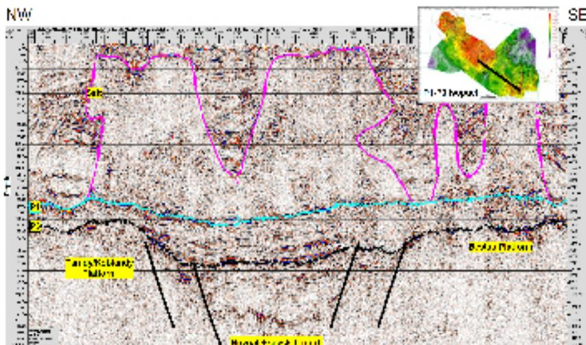
**Figure 1. Seismic profile along the OTG-06-20 line through the Kobylanda-Tamdy tectonic step - Novoalekseevsky trough - Bestau uplift**
