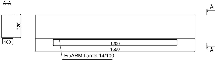
**Fig. 3 — Reinforcement structure of the reinforced concrete beam with FibARM Lamel 14/100**
