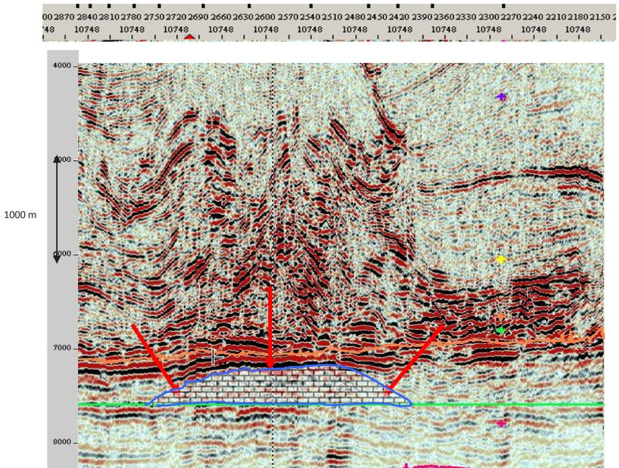
**Figure 3. The structure of Kobylandy. Crossline 10652 seismic section showing prospective reef construction**
