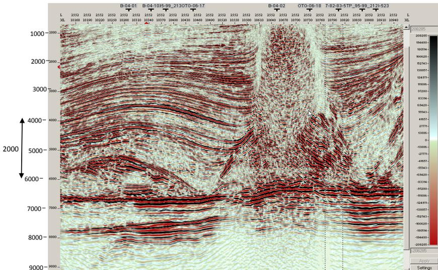
**Figure. 4 Structure of Kobylandy. Inline 2552 seismic section showing deposition of the Middle Devonian complex**
