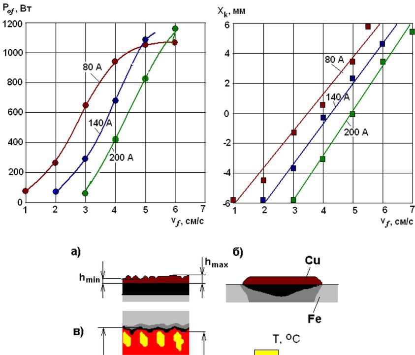
Fig. 3. The dependence of the power  $P_{of}$ , absorbed by the wire from the plasma torch of the main arc (a) and the displacement  $X_k$  of the drop on the wire relative to the axis of the plasma torch on the wire feed speed  $v_f$  for different values of the additional arc current (b) [1]:  $B_{max}$  and  $B_{min}$  are the maximum and minimum surfacing width ;  $h_{max}$  and  $h_{min}$  are the maximum and minimum height of the deposited layer.
