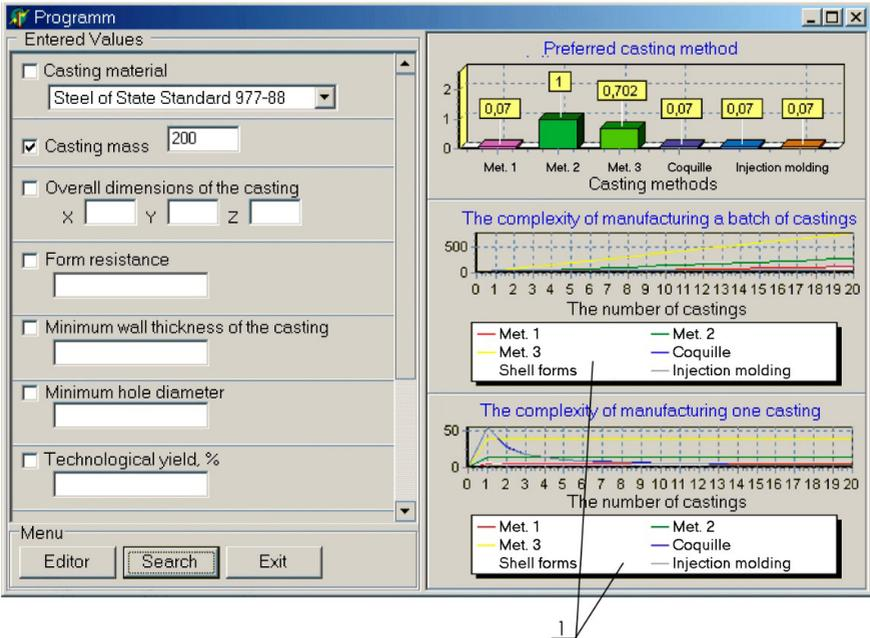
Figure 2. Analysis input window with chart legend enabled where 1 is legend chart
